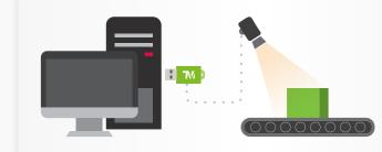
□TM AI+<sup>TM</sup> AOI Edgecan be installed on any personal/industrial computer at production lines. After connecting the computer to external camera, the user can perform vision tasks like item recognition, image enhancement and measurement through TMvision™.
